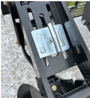
Figure 3.45 Mechanical Spring Packer
