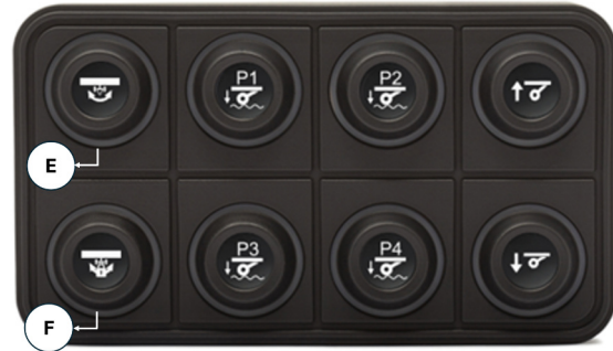
Figure 3.35 Hitch Control Keypad
