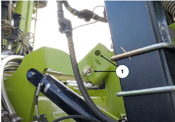
Figure 3.41 Location of Wing Lock Pins
